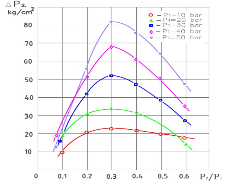
Figure 2. Dependence diagram of pressure peak-to-peak motion from cavitation parameter
