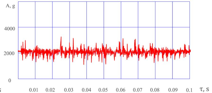
Figure 2. Oscillogram of vibration acceleration at the rock-cutting tool for the inlet pressure  $P_1 = 41$  bar,  $P_2 / P_1 = 0.17$  the cavitation parameter and 450 Hz frequency.
