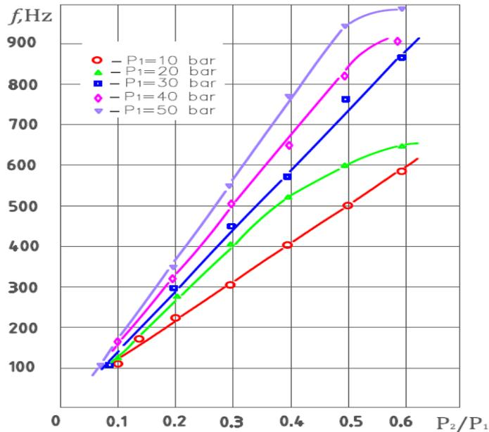
Figure1. Dependence diagram of frequency from cavitation parameter
