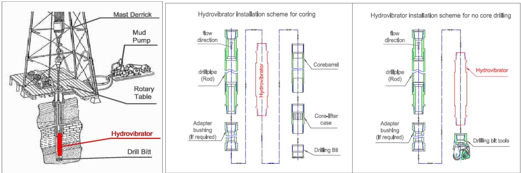
The high-frequency cavitating hydrovibrator is installed to the drilling liner and placed in a vertical or horizontal well.
