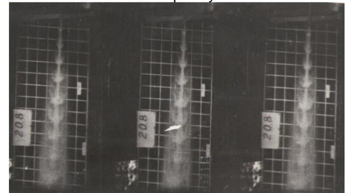
Picture 1. The fragment of high-speed video filming (2980 frame per second) demonstrates the pulsing flow at the outlet of hydrovibrator.
