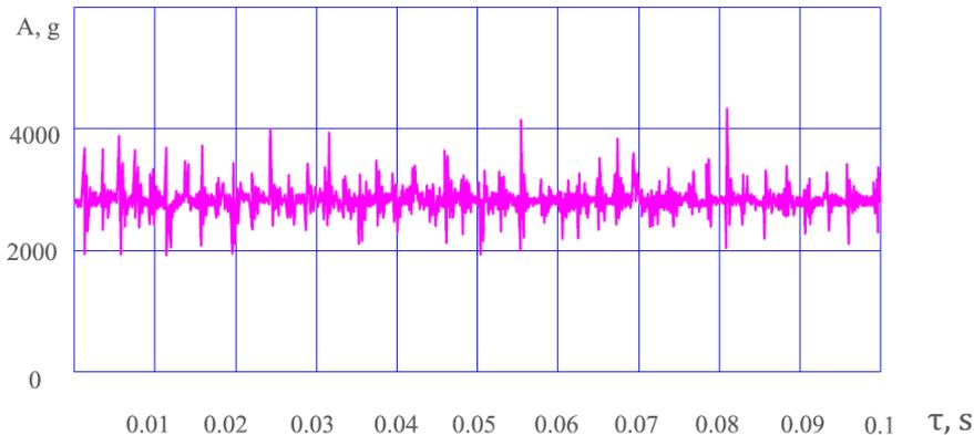
Figure 1. Oscillogram of vibration acceleration at the section of hydrovibrator for the inlet pressure  $P_1 = 41$  bar,  $P_2 / P_1 = 0.17$  the cavitation parameter and 450 Hz frequency.
