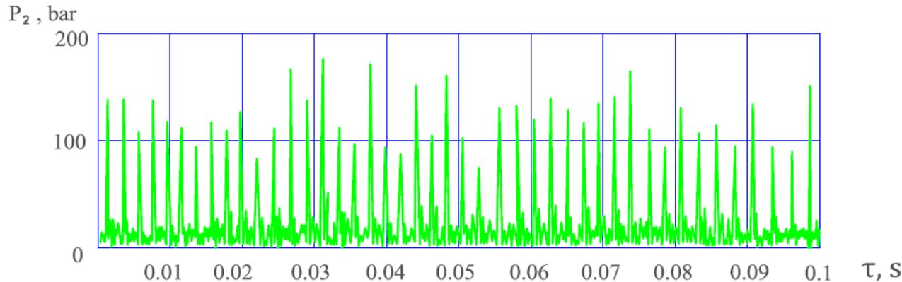
Oscillogram fragment of pressure oscillations  $P_2$  at the outlet of the hydrovibrator for input pressure  $P_1 = 41$  bar and  $P_2 / P_1 = 0,17$  the cavitation parameter
