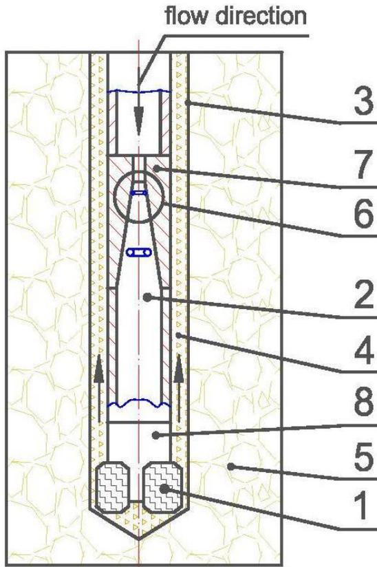
Schematic representation of the vibration-rotational drilling using cavitation hydrovibrator
